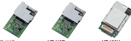
UT-109R Non-rolling type voice scrambler for analog mode UT-110R Rolling type voice scrambler for analog mode UT-126H, UT-126HL IDAS NXDN digital unit
