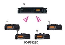
The IC-F5123D series allows you to call individual or group users. The radio automatically sends own ID number when the PTT button is held down. The alias name or individual/group ID is displayed on the LCD while receiving a message allowing you to identify who is calling.
